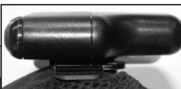
PowerBox can easily be removed for charging or replaced with a fully charged unit to allow for extended shift patterns. Slide the PowerBox unit upwards, disengaging from the moulded loops.
